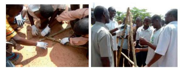
Measure the middle point on each stick and nail the cross bar across the two. Make it relative to one's size. Make a middle point on the cross bar, tie the string from the top onto the heavy object. The string must pass through the middle point – if it doesn't you have not made it properly. Make your contours using the A frame.
