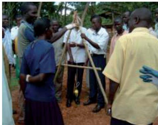
Keeping one leg of the A frame on the floor, move the other leg round along your plot. When the string passes through the middle point, mark where the 2<sup>nd</sup> leg is. Then keep that leg on the floor, and move the first leg of the A frame around. When the string passes through the middle point, mark again. And so on..... You will soon end up with a row of markers
